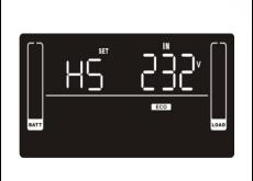
For 100/110/115/120/127 VAC models, the setting range is from +3V to +12V of the nominal voltage (Default: +6V).
